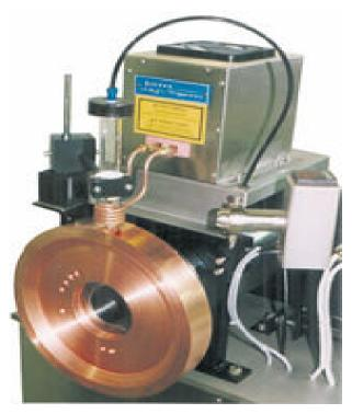
Fig. 4.2 Melt-spinning Mechine
