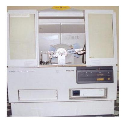
Fig.4.8 A PHILIPS PW3040 X'Pert PRO X-ray diffractometer.
