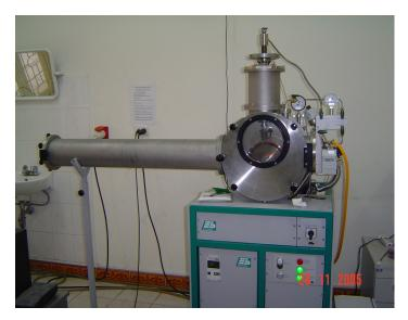
Fig.4.1 Vacuum arc melting machine
