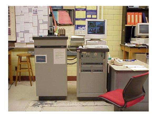
Fig. 4.13 SQUID Magnetometer.
