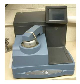
Fig. 4.4 Differential Scanning Calorimeter (TA Instruments Q100).
